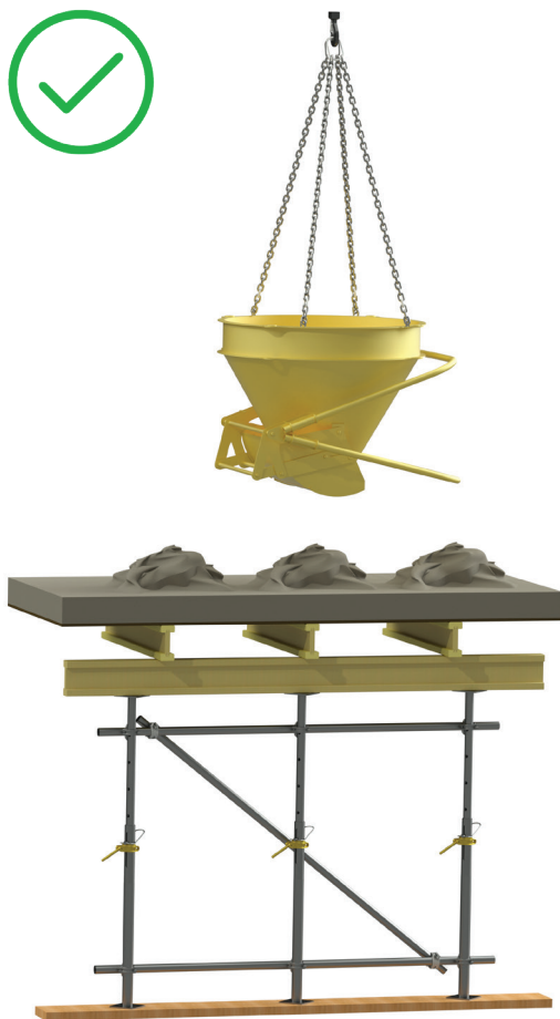
Apply uniform loads, to prevent prop buckling
