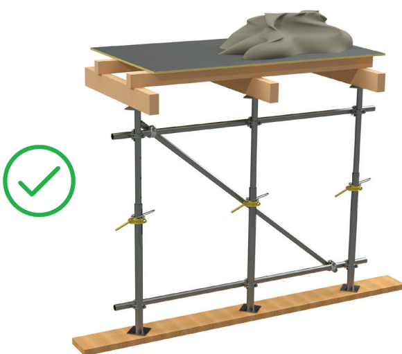
Using bracing for falsework stability
