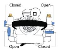
Position of the CLEARFLOW pump valves when dumping
