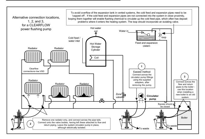
The connection point for the Clearflow pump may vary depending on the system to be cleaned, and the availability of suitable connection points.
