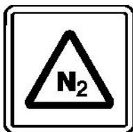
The accumulator must only be charged with Nitrogen.
