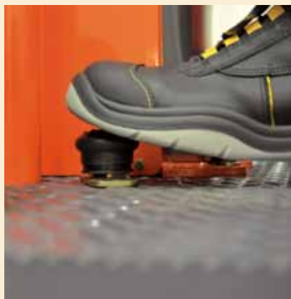
Water and additive sprinkling constant control can be activated via a foot switch.
