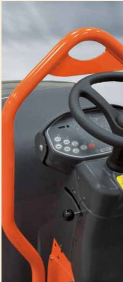
An ergonomically-designed grab handle in the center of the machine allows quick and safe access. On the HD 8 - 12, it also serves as the central suspension point for lifting the machine.
