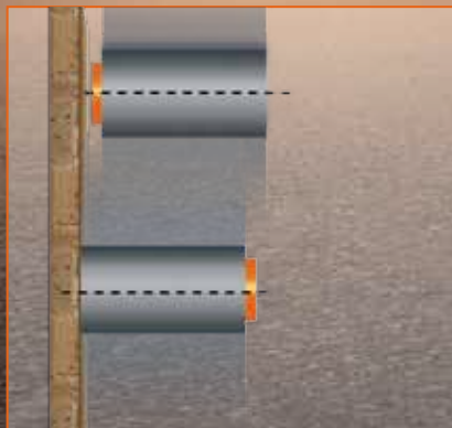
Single-side drum support on the HD 8 and HD 10C models ensures compaction up to the edge.
