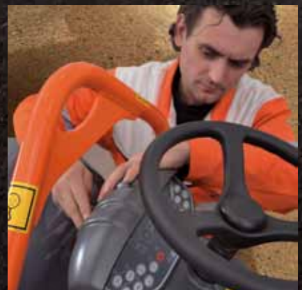
The protective cover prevents unauthorized operation and deters vandalism.
