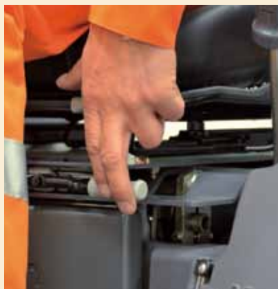
The driver's seat can be effortlessly shifted from one side to the other (HD 10 – HD 14).
