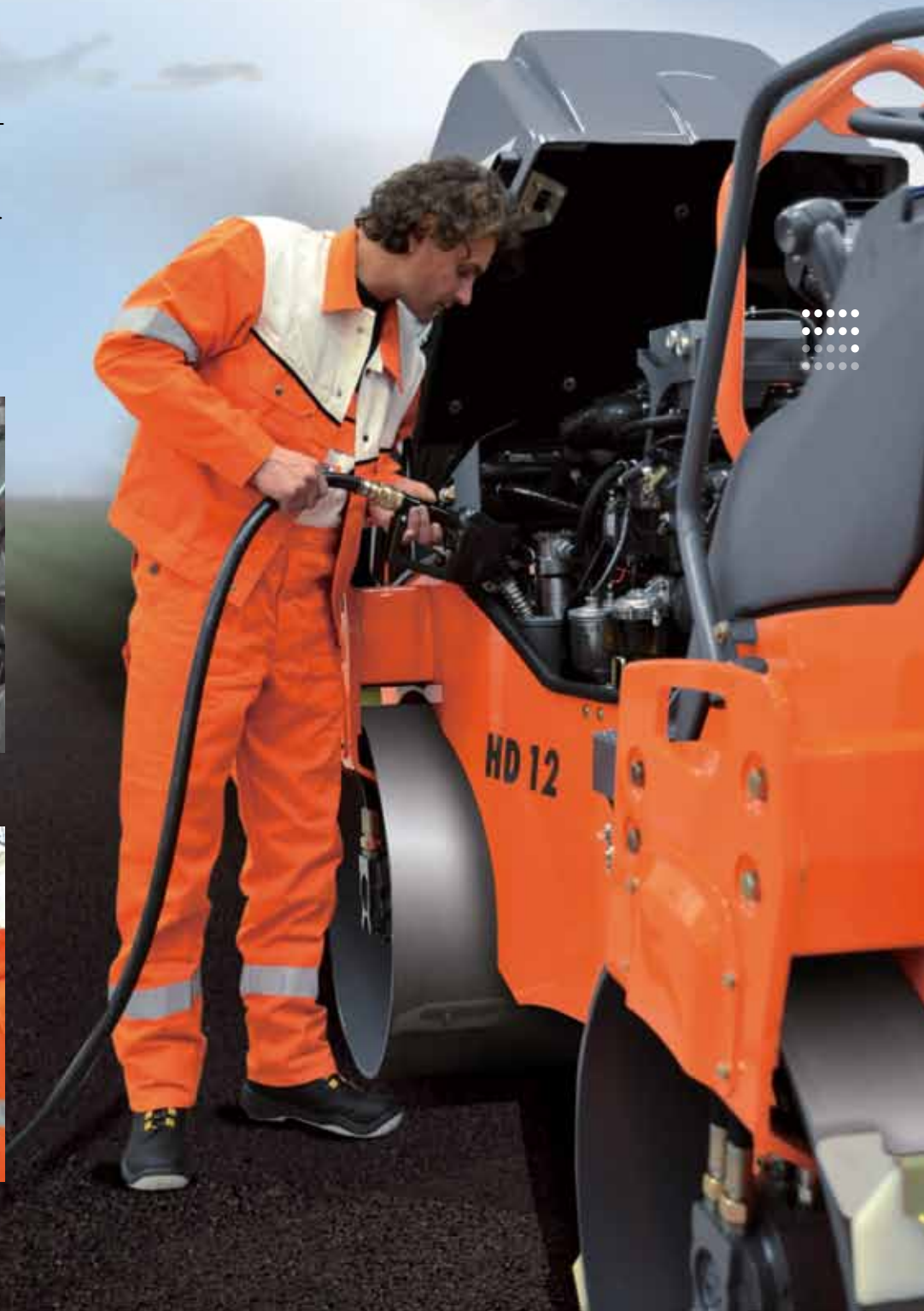
Inspection in a matter of seconds: the large-sized, self-cleaning water filter is located directly behind the tank lock.
