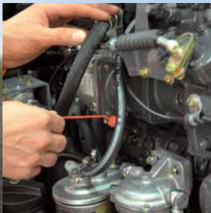
Easily accessible: the well-positioned engine oil dipstick.
