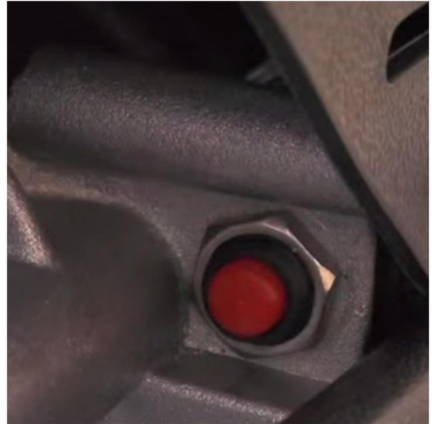
There may be instances your compressor will overheat. If it cuts out, this is a safety feature to protect you and your compressor. Leave this compressor for a good while until you reset it. If the compressor turns off again on re-set you should not keep running it as it may be damaged and the system may be unsafe.
