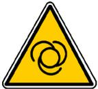
Risk of accidental start-up. The compressor could start automatically in the event of a power cut and subsequent reset. Do not carry the compressor while it is connected to the power source, or when the tank is filled with compressed air.
