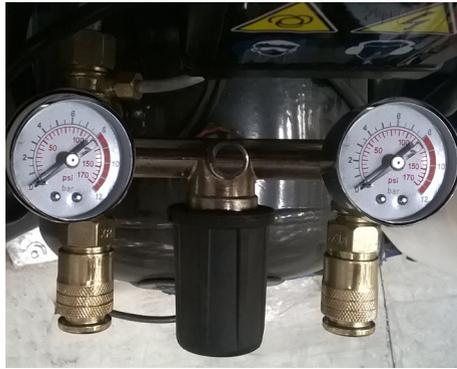
2. The output pressure of compressed air can be adjusted by the regulating valve. Grip the regulation valve knob and turn it clockwise to increase the pressure.
