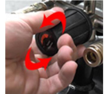
5. Once the compressor is vented, remove any condensation from inside the tank by unscrewing the bleed nipple.
